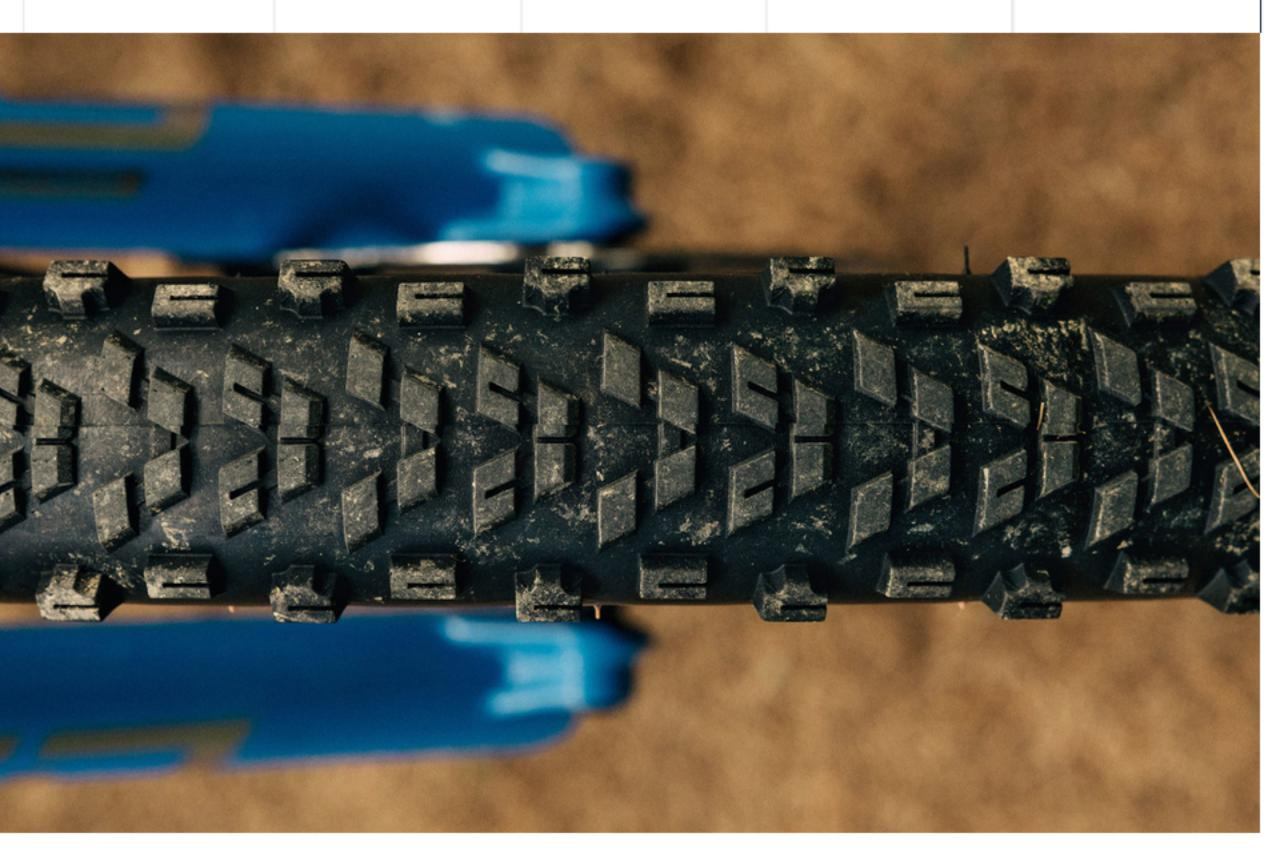
The Wyrm's large volume provides the advantages of a larger tyre without the drawbacks. It allows for lower tyre pressure, resulting in increased flexibility, deformation, and improved traction, braking, and cornering ability.
